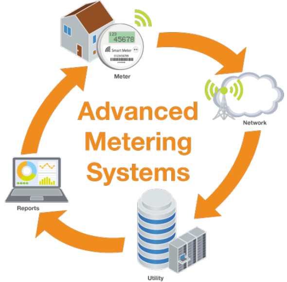
Advanced Metering Infrastructure (AMI)
